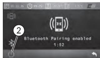
Activate and deactivate the Bluetooth connection by means of the On/Off function ② in the submenu.
