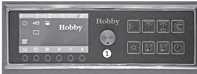
The system consists of control electronics, a TFT control panel with a keypad and several peripheral panels. It enables you to operate the different lights and several 230 V devices. Furthermore, various kinds of information and measured values are shown on the TFT display.
