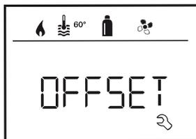
The temperature sensor for the heating can be individually adjusted to the size of the vehicle. The offset can be set in increments of 1°C within a range of -5°C to +5°C.
